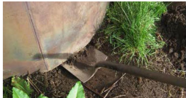
Creating a passage for air flow under a biochar kiln.
