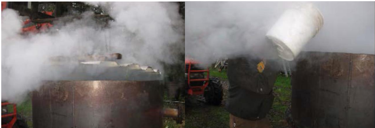
The lid method (left) or the dousing method (right) are both ways to extinguish biochar fire. Photos: Steve Bensel
