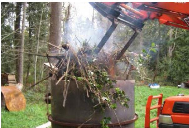
Adding woody biomass to a biochar kiln. Photo: Steve Bensel
