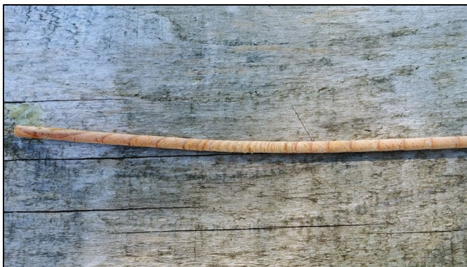
Consistent 1/4" growth rings on 50 year old Douglas-fir.
