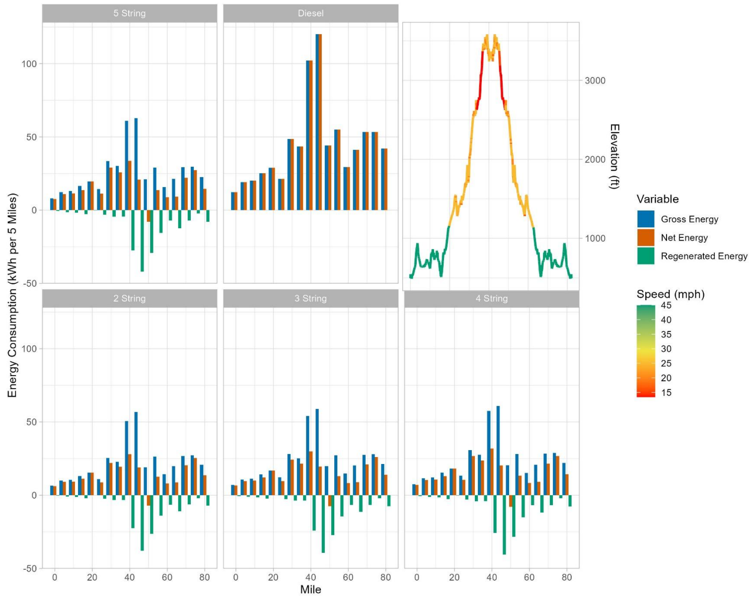
Figure D4: Round trip elevation, speed and energy cost (kWh) bar charts at 5mi intervals for the Scott Turner Road from the Vener mill for every vehicle configuration
