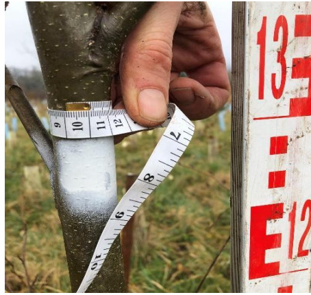
Figure 11 (far left): Using a straight edge and spray paint to create a sharp and re-samplable line for diameter measurements
